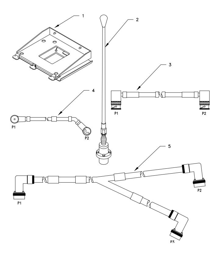
Figure 4-1. MK-2867/VRC Illustrated Parts List
